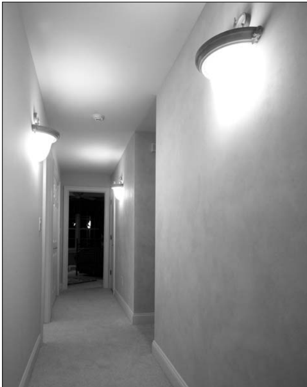
Traditional incandescent fixtures can now be replaced with pin-based compact fluorescent light fixtures. A range of residential styles are now being offered.
