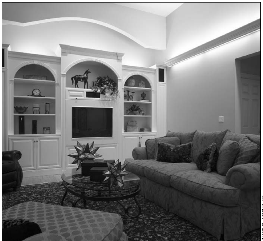
A custom-built valance directs light upward and downward ( top ), and is coordinated with the materials and mounting location of other cabinetry ( bottom ).
