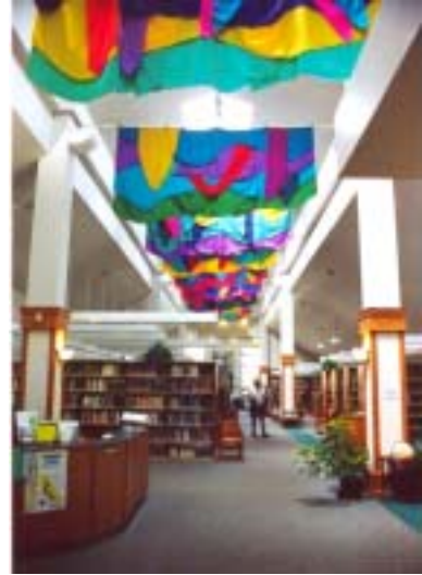
Cameron Park Library, Peter Wolfe Architect. A skylit library provides a stimulating yet peaceful environment. Colorful banners enliven the space while blocking glare from the skylights and helping to diffuse the daylight. Photo courtesy Lisa Heschang.
