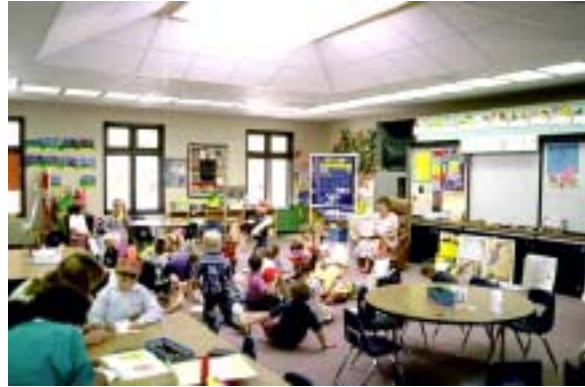
Classroom with central skylight and splayed light well walls. Photo courtesy PJHM Architects
