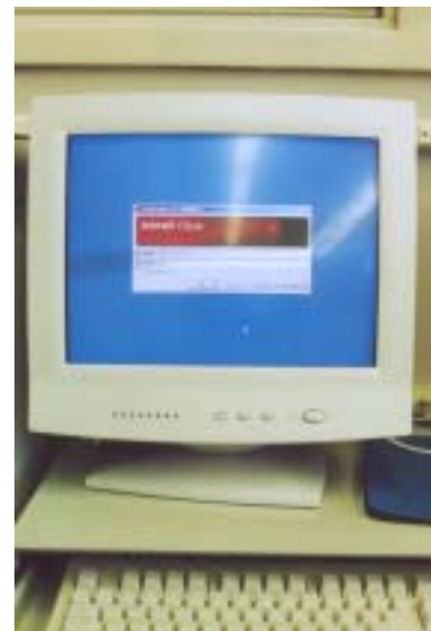
Reflections of luminaires in computer screens can cause veiling glare. Careful lighting and daylighting design avoids these problems. Photo courtesy Lisa Heschong.
