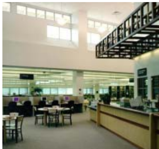
Sidelighting: Library receives daylight from two sidelighting strategies: 1) view windows at perimeter, and 2) high clerestories that bring daylight into the center of the space.
