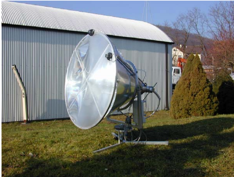
Figure 4: A SOLUX-collector without the protecting acrylic dome [Colsman-Freyberger, 2002].
