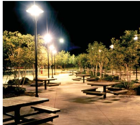
Close spacing of low-output luminaires reduces glare and provides comfortable lighting for faces.
