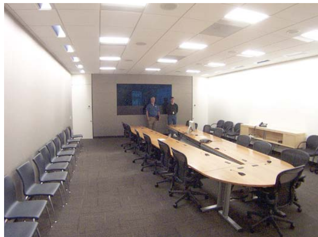
Be sure that ceiling luminaires are outside of the camera's view in videoconferencing rooms.
