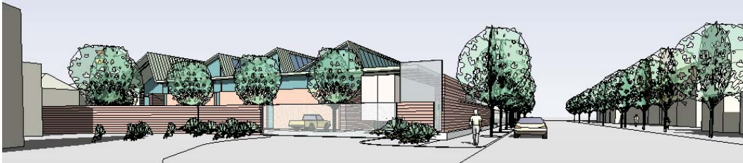
North-facing monitors enable daylight to be the primary light source for the warehousing functions at Sunrise Yards, a current DDC project in Queens, NY.
