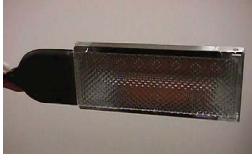
Figure 12: The prototype lamp head with diffuser to even out the light distribution.
