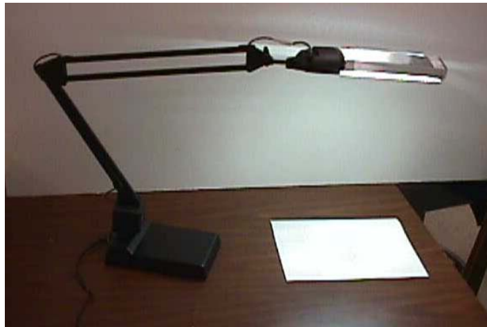
Figure 9: Prototype #1, LED task lamp
