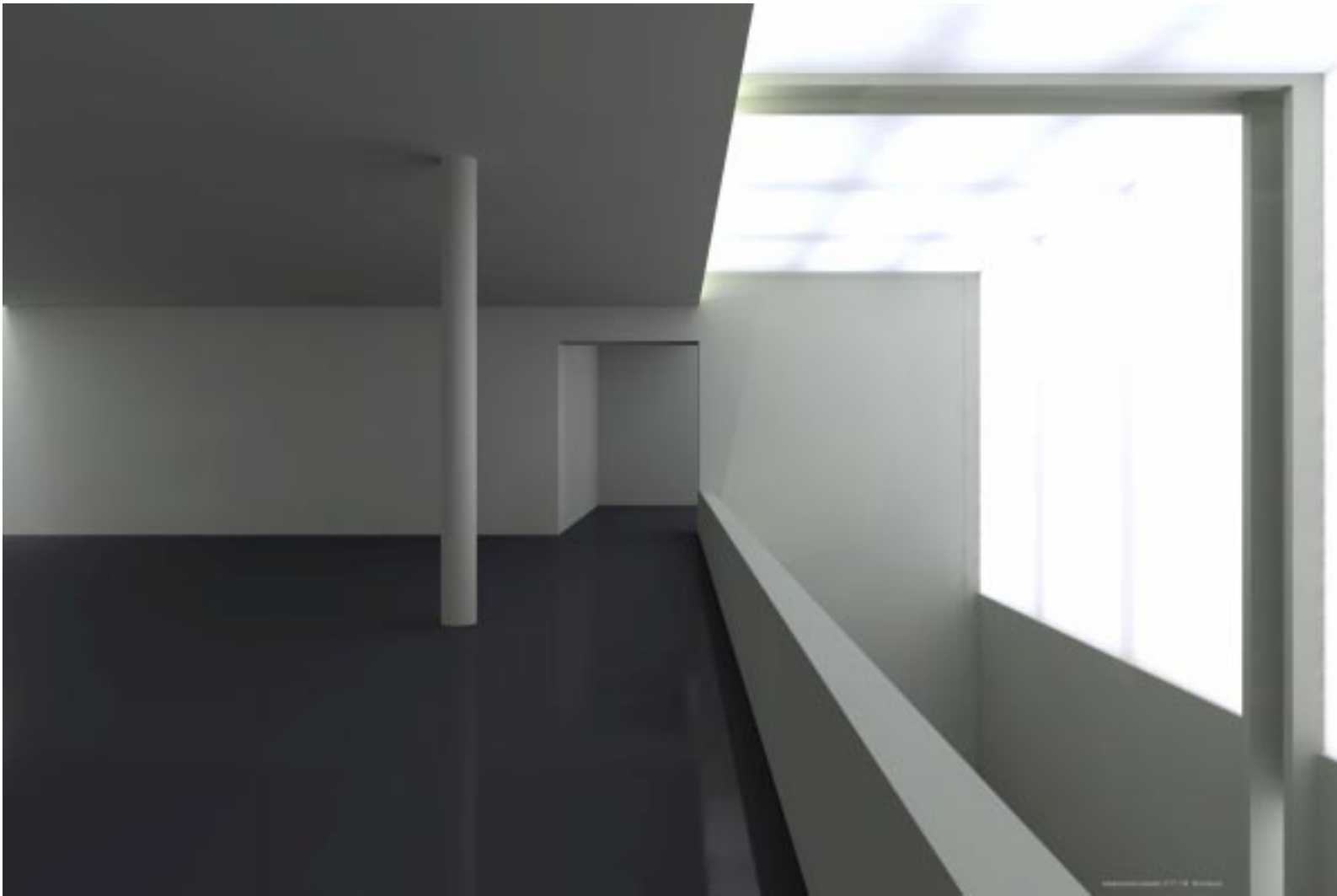
Fig. 1. A daylighting simulation of the two-story gallery of The Art Museum of Estonia. Exterior conditions: horizontal illuminance 10 klx, vertical illuminance 5 klx.
