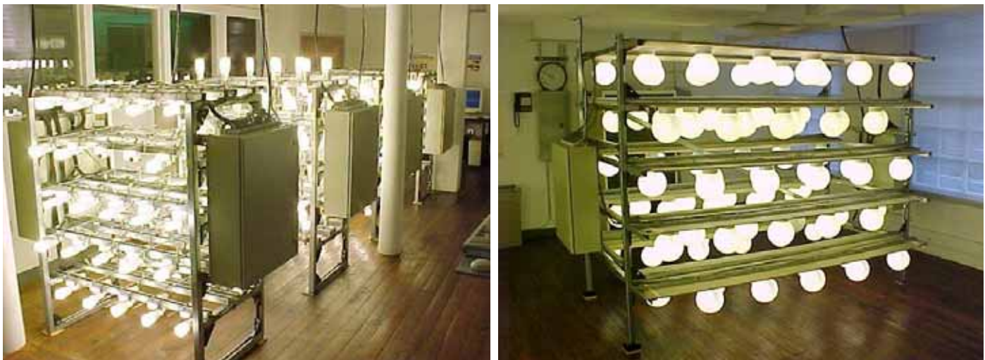
Figure 1. Lamp testing racks for horizontal, base-up and base-down conditions (left), and for enclosed conditions (right).
