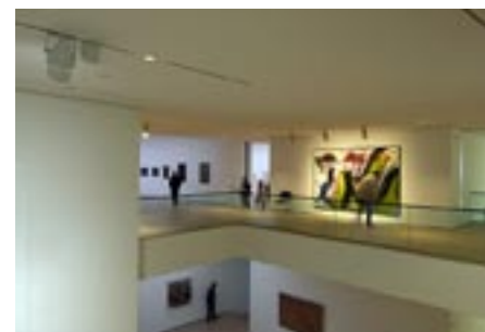
Regardless of whether it is large-format advertising surfaces or walls with artworks in museums that are to be illuminated – uniform, vertical illuminance is an effective concept to illuminate walls and objects.
