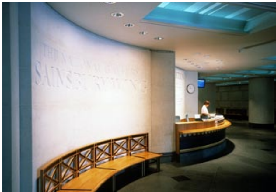
Wallwashing aids orientation in entrance areas: visitors understand the structure of a room faster and assimilate important information quicker. Particular details on walls such as inscriptions become even more noticeable.
