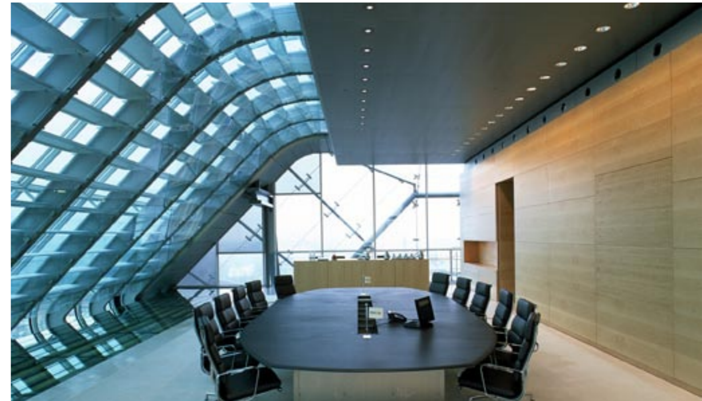
Wall lighting in the daytime reduces the contrast of bright facades and room walls. At night, the even lighting of wall areas ensures a bright spatial impression is maintained.
