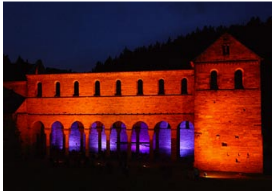
The colour contrast of cold and warm hues gives a festival in the ruins a most attractive setting. Many luminaires allow the light colour to be changed using colour filters.
