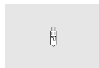
Low-voltage halogen capsule lamps and tungsten halogen lamps provide brilliant light and, thanks to their continuous spectrum, perfect colour rendition.
