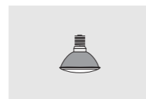
Parabolic aluminised reflector lamps and halogen parabolic reflector lamps are renowned for their brilliant light and very good colour rendition. The parabolic reflector makes the first contribution to harnessing the beam.
