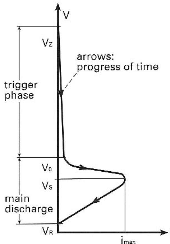
The impedance characteristic (anode voltage  $V$  versus discharge current  $i$ ) features the same form for all flash discharges. Its slope represents the characteristic of the discharge (increasing/decreasing).
