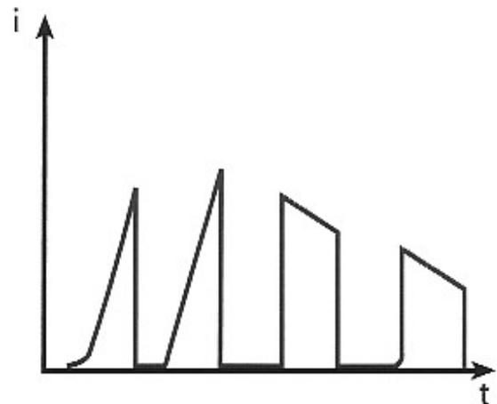
The IGBT offers high peak current, high frequency switching with very low loss and simple driving circuit. This concept is ideal for discharge control of flashtubes. The IGBT also operates the tube's trigger circuit. All pulse patterns,
