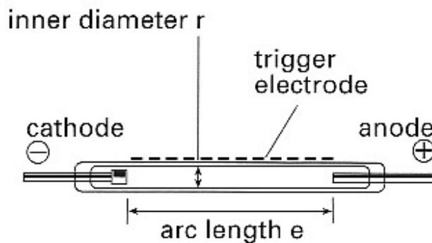
*Schematic drawing of a flashtube*
