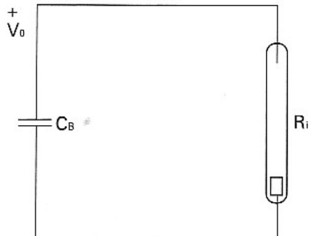
After peak current  $i_{\max}$  has been reached, an almost exponential discharge of CB takes place, since the internal resistance  $R_i$  of the tube remains constant. The time constant  $T=R_i C_B$  is a measure for the flash duration ( $\sim 1/3$  value).  $V_0$  ranges often between 200-400V. This is due to the electric strength of the electrolytic photoflash capacitors.
