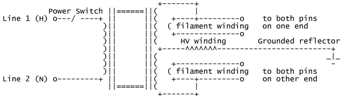
Loose magnetic coupling in the ballast core results in leakage inductance for current limiting.
