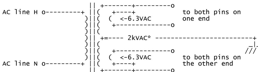
\*The high voltage winding of the secondary is on a branch magnetic circuit that limits the output current to the mercury discharge. Most of the 48" 40W "shop light" type of bulbs use this. Open circuit voltage will be in the kilovolt range, while the voltage across a lighted tube will be somewhat less than that and \*exceedingly\* non-sinusoidal.
