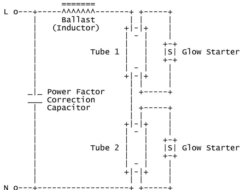
Note that starters for a 230 VAC two tube fixture may NOT be the same as those for a 230 VAC single tube fixture. Installing single tube starters in a two tube fixture may result in no action at all since their breakdown voltage may be too high. Doing the reverse may result in damage.
