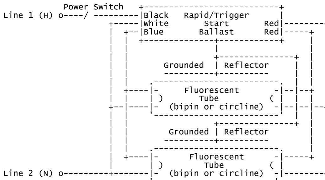
Note: The interlock normally present on most rapid/trigger start fixtures have been removed to permit one lamp to operate if other is removed.
