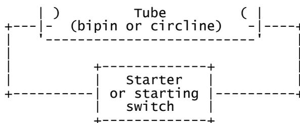
Where a three position switch (OFF-ON-START) is used to control the fixture (e.g., those circular magnifier lamps), there will be two pairs of contacts: One pair (Power) is connected in the ON and START positions, and the other (Start) is connected only in the START position. They are isolated from each-other.
